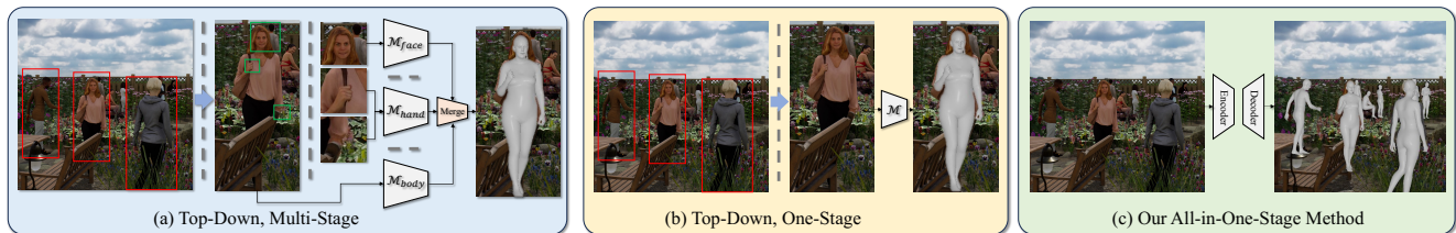
Figure 1. A comparison of existing methods in EHPS. (a) Top-down, multi-stage methods typically use detectors to detect humans, then use different networks to regress body parts on cropped images. (b) Top-down, one-stage methods use only one network for regression but still require detectors and rely on the cropped image. (c) Our all-in-one-stage pipeline, end-to-end human detection, and regression on full frame.
